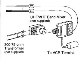
If your TV has both post and plug-type VHF terminals, the post connection is recommended to minimize signal loss.
