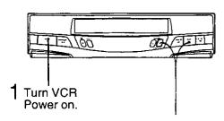
2 Press and hold both PLAY and CHANNEL ▲ on the VCR for more than 5 seconds.
